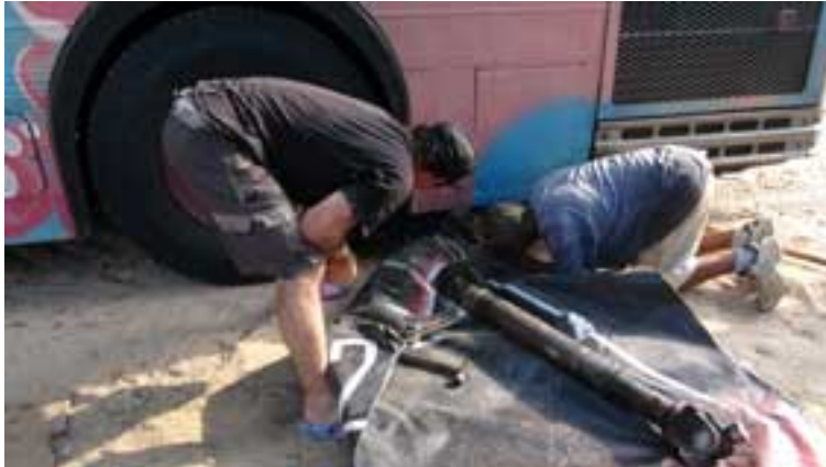
The Drive Line broke the Bus stopped.
